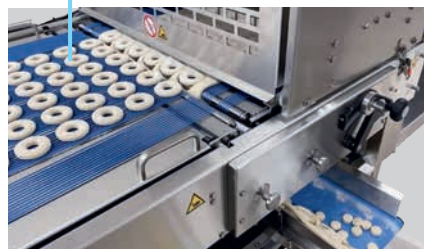
4 Automatic removal of the dough scraps
