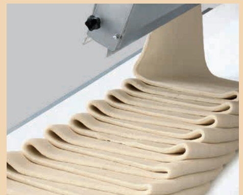
Use a RONDO MLC modular laminating line to automate the production of puff-pastry and Danish dough products with continuous feed of the Starline.
